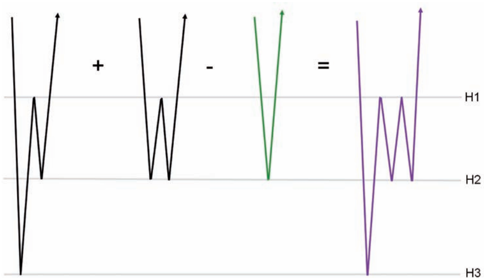
Fig. 2. The three diagrams on the left represent the subevents combined to predict the internal multiple on the right. In this example, the two internal multiples (black) with traveltimes t_{312} and t_{212} are convolved together and crosscorrelated with the generating primary (green) with traveltimes t_2 . The combination results in the second-order internal multiple (purple) with traveltimes t_{31212} .
