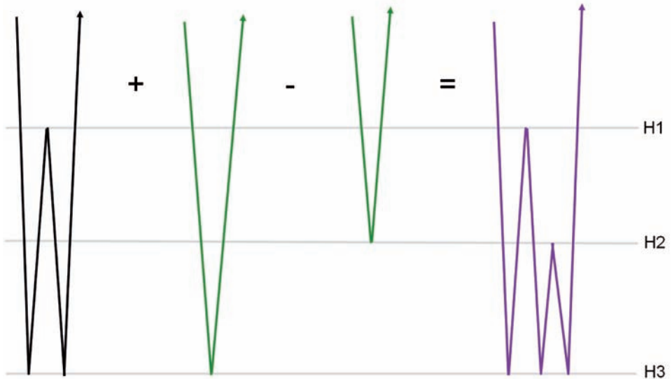
Fig. 3. Example of an internal multiple predicted using the generator P_2 . Observe that only the generator contains explicitly an instance of traveltime t_2 , but the combination still produces the traveltime of a true internal multiple, (t_{31323} = 3t_3 - t_1 - t_2) .
